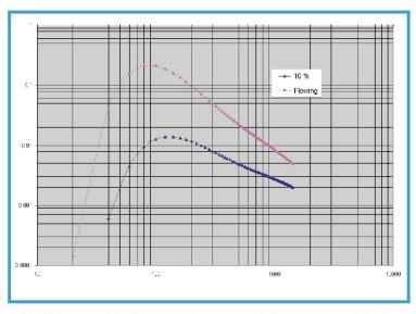
Absolute efficiency registration comparison curves during gamma-emissioning sample positioning inside and outside detector
